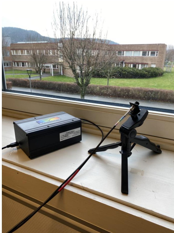
Figure 2.5 The set up with spectrometer and sensor.
